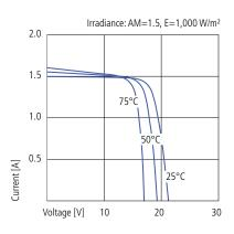
Current-voltage characteristics of PV module LORENTZ LA20-12S at various cell temperatures.
