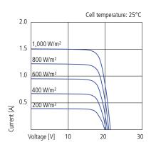
Current-voltage characteristics of PV module LORENTZ LA20-12S at various irradiation levels.
